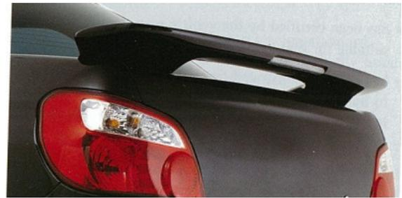
Rear spoilers must be within the body shape/outline of the mounting surface (for example, the boot outline). The minimum thickness of end plates is 4mm and they must be free of sharp edges or corners.
